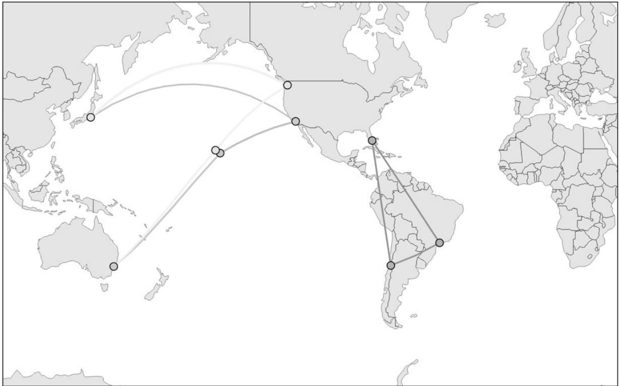
Figure 5: Topology map showing average bandwidth for the backbones and exchange points. Darker lines and nodes represent higher bandwidth.
