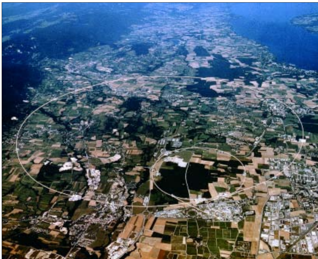
Figure 2. An aerial view of CERN. The Large Hadron Collider (LHC) ring is 27 km in circumference and provides two counter-rotating, 7 TeV proton beams to collide in the middle of the detectors.
