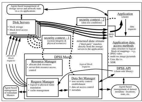
Figure 7 Distributed-Parallel Storage System architecture.
