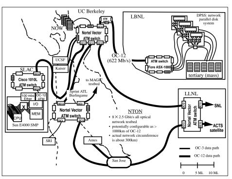
Figure 9 The LBNL - NTON - SLAC high-speed, data intensive distributed computing experiment.
