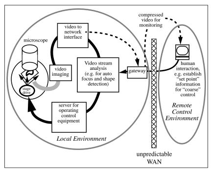
Figure 5 Remote, semi-autonomous, dynamic experiment operation architecture.
